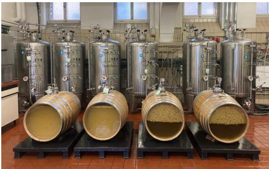
Figure 2 Photo of the 8 variants during alcoholic fermentation: in the background are the stainless steel tanks and in the foreground the barrique barrels with VBUNG® technology.
